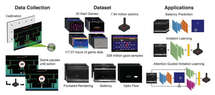
Figure 1: Project schematic for the Atari-HEAD dataset.
