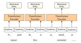
Figure 3: Illustration of how we leverage a *transformer encoder* to incorporate subword embeddings into word-level representations. The parameters in the *transformer encoder* are shared for all subword embeddings.
