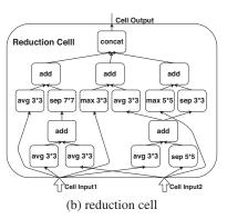
Figure 6: the normal and reduction cells that yield the highest accuracy in the search.
