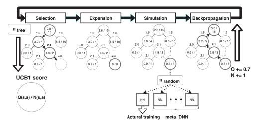
Figure 2: Overview of AlphaX search procedures: explanations of four steps are in sec.3.2.
