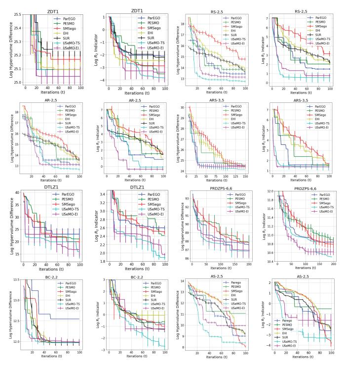
Figure 2: Results of different multi-objective BO algorithms including USeMO on synthetic benchmarks. The log of the hypervolume difference and log of  $R_2$  Indicator are shown with different number of function evaluations (iterations). The mean and variance of 10 different runs are plotted. The tile of each figure refers to the benchmark name defined in Table 1.
