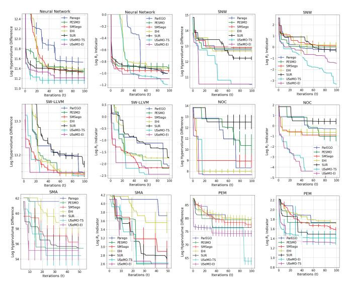
Figure 3: Results of different multi-objective BO algorithms including USeMO on real-world benchmarks. The log of the hypervolume difference and Log  $R_2$  Indicator are shown with different number of function evaluations (iterations). The mean and variance of 10 different runs are plotted. The tile of each figure refers to the name of real-world benchmarks.
