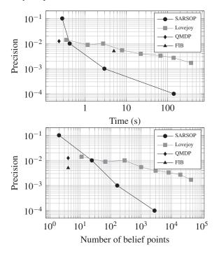
Figure 2: Illustration of the time precision trade-off for different algorithms providing upper bounds on the value function in a POMDP. Lovejoy is the algorithm used by Norman, Parker, and Zou. To compute the precision, we used the lower bound computed using SARSOP as a reference. The experiments are carried on a  $3 \times 3$  partially observable grid world domain.
