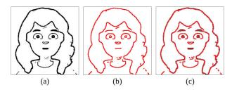
Figure 11: Example of pixel-coordinates extraction. (a) The avatar sketch; (b) Simulated drawing using extracted pixel-coordinates; (c) Overlay of (a) and (b).
