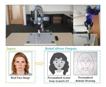
Figure 1: Top: the robot performing the drawing; Bottom: the generated personalized avatar and the drawing result.
