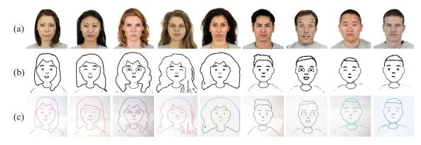
Figure 14: Results of the integrated tests, where (a) are the real face images, (b) are the corresponding cartoon avatars generated by AvatarGAN after coherent contour generation, and (c) are the marker-on-whiteboard drawings finished by the robotic arm.
