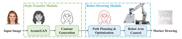
Figure 2: Pipeline of the RoboCoDraw System.
