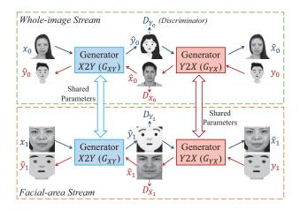
Figure 4: The structure of AvatarGAN, which consists of two translation streams. The whole-image stream performs ordinary style translation between real faces and avatars, while the facial-area stream focuses on learning facial feature mappings between the two domains.
