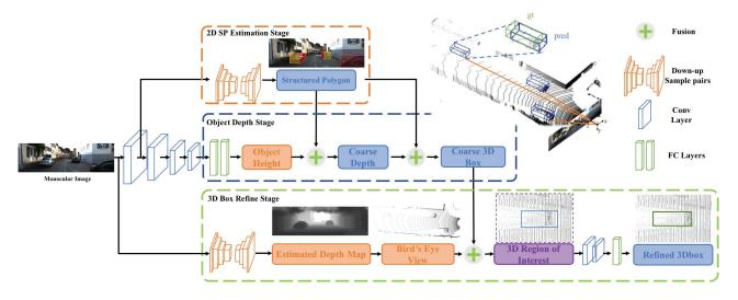
Figure 2: The overall framework (*Decoupled-3D*) decouples the monocular 3D object detection problem into sub-tasks. The overall network consists of three parts. (Top row) The 2D structured polygons are generated with a stacked hourglass network. (Middle row) Object depth stage utilizes 3D object height as a prior to recover the missing depth of the object. (Bottom row) 3D box refine stage rectifies coarse 3D boxes using bird's eye view features in 3D-ROIs. Best viewed in color.
