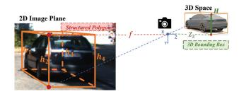
Figure 5: Height-Guided Depth Estimation. Combine object height H and corresponding pixel value h to estimate object depth. Best viewed in color.
