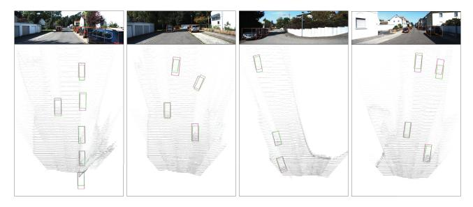
Figure 7: Qualitative Results. Top: structured polygons. Bottom: 3D bounding boxes in bird's eye view. Camera center is located at bottom center. Predicted 3D bounding boxes are drawn in pink, while ground truths are in green. Best viewed in color.
