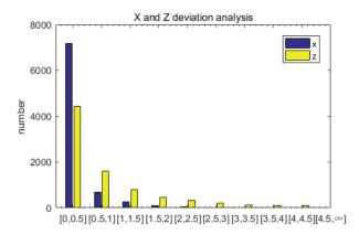
Figure 8: Deviation analysis of X and Z. The figure shows the number of absolute deviation of X and Z of the coarse boxes compared with ground-truth boxes in different interval segments. Best viewed in color.
