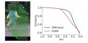
Figure 4: Detection sensitivity analysis. (Left) Sequence of boxes (marked in green) for calculating the similarities to the perfectly-aligned first box (marked in red). (**Right**) Similarity vs. IoU for the box sequence. Our method is better at assigning lower similarities to false detections (IoU< 0.5).
