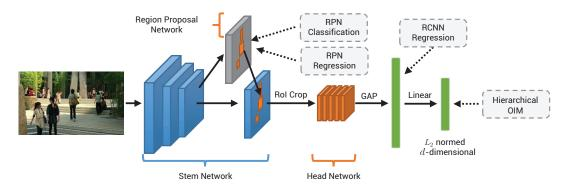
Figure 2: Overview of our framework. Our network is based on Faster R-CNN (Ren et al. 2017) with a ResNet-50 (He et al. 2016) backbone. An extra  $L_2$ -normalized linear projection layer is appended for person embedding generation. We remove the second-stage classification loss of the original Faster R-CNN and integrate its functionality into our HOIM loss.
