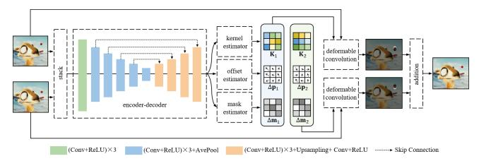
Figure 3: Illustration of the architecture of our proposed DSepConv network. The encoder-decoder architecture extracts features, which are given to three sub-modules to estimate separable kernels, offsets and masks for each output pixel. The input frames are then convolved adaptively with deformable convolution described in Eq. (3) and (4).
