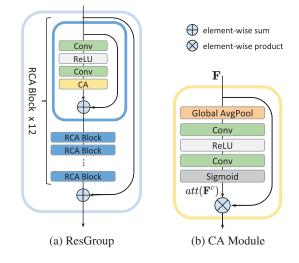
Figure 4: Illustration of ResGroup and CA module.
