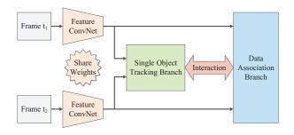
Figure 2: The overall architecture of the proposed DASOT-Net. It consists of three modules: feature ConvNet, data association branch and single object tracking branch. These two branches interact with each other during joint training.
