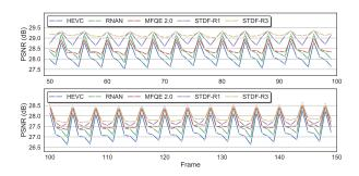
Figure 6: PSNR curves of 2 test sequences at QP 37. Top: *BQSquare*. Bottom: *PartyScene*.
