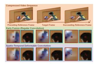
Figure 3: Visualization of EF and our STDC. Herein, red points represent the sampling positions of  $3\times3$  convolution window centered at green points. The STDC can adapt to both large temporal motion (ball) and the small one (head), and accordingly captures the relevant context for quality enhancement.
