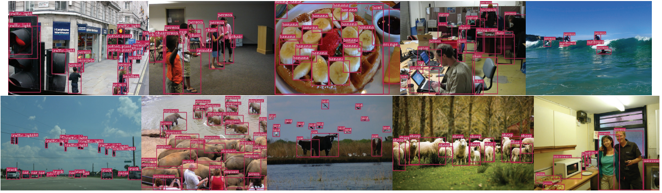
Figure 4: Qualitative examples of our EHSOD trained on 30% fully-supervised COCO data. EHSOD can detect tiny and occlusion objects due to the help of image-level information.
