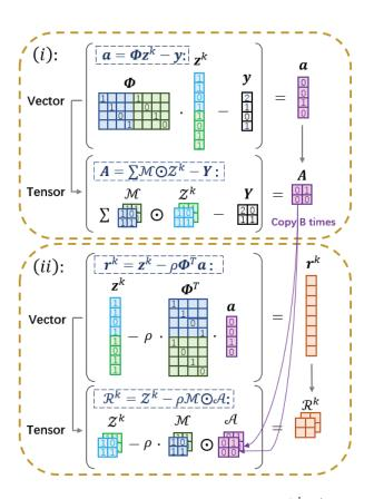
Figure 4: Illustration of tensor calculations of  $\mathcal{R}^k$ . A in the first step is the middle result of calculation. In the second step A is copied B times to form tensor A in third dimension.
