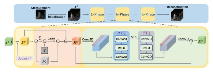
Figure 3: The proposed *Tensor FISTA-Net*. The upper part is the data flow in *Tensor FISTA-Net*, containing K phases. The bottom part is the detailed structure of a phase. Gray arrows denote the data flow.
