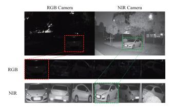
Figure 1: Examples of images captured by RGB and NIR cameras from six camera views. Middle: the RGB images of six camera views. Bottom: the corresponding NIR images.
