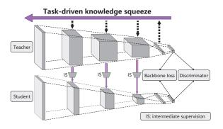
Figure 1: The overview of proposed Hierarchical Knowledge Squeezed Adversarial Network Compression (HK-SANC) via intermediate supervision.
