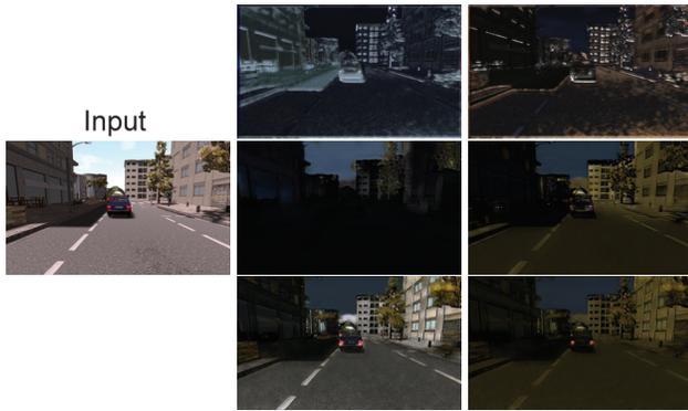
Figure 3: SYNTHIA day-to-night transformation results generated by GANs trained with SYNTHIA given different random vectors: 1st row: results of AugCGAN; 2nd row: results of MUNIT; 3rd row: results of this work.
