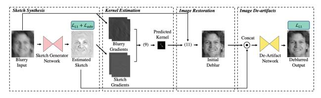
Figure 2: Overview of our network. Blurry inputs are fed into a sketch generator network to predict sketches supervised by adversarial and content losses. Then, given the gradients of blurry inputs and sketches, blur kernels are estimated by (9). Afterward, initial deblurred images are restored via (11). To further suppress artifacts, the final deblurred results are obtained by a de-artifact network.
