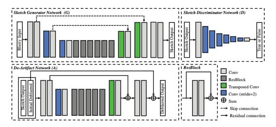
Figure 3: Structure of the sub-networks. Sketch Generator Network contains 10 convolutional layers, 2 transposed convolutional layers, 6 residual blocks, and 2 skip connections. Sketch Discriminator Network is identical to *PatchGAN*. De-Artifacts Network contains 7 convolutional layers, 1 transposed convolutional layer, 5 residual blocks, and 2 residual connections.
