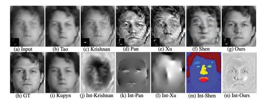
Figure 1: A challenging case for face image deblurring. "Int" denotes the intermediate structure or face parsing of its corresponding algorithm. The bottom left corners of (a) and (c)(d)(e)(g) are the ground truth blur kernel and the estimated ones, respectively. The proposed method generates a sketch (n) with semantic structures and restores a higher-quality image (g) via an end-to-end network based on the conventional deblurring process.
