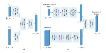
Figure 2: Illustration of two kinds of fusion blocks. (a) FBv1, (b) FBv2. The kernel sizes (along with channels if necessary) and strides of operators are shown. The strides are (1,1,1) where not specified. Best viewed in color.
