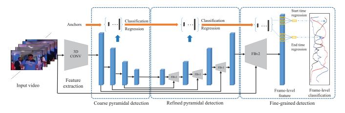
Figure 1: Architecture of our proposed progressive boundary refinement network (PBRNet). PBRNet belongs to the one-stage detectors and mainly consists of three key components: coarse pyramidal detection, refined pyramidal detection and fine-grained detection. The three components sequentially refine the boundaries of action candidates accompanied by the enhancement of features. Best viewed in color.
