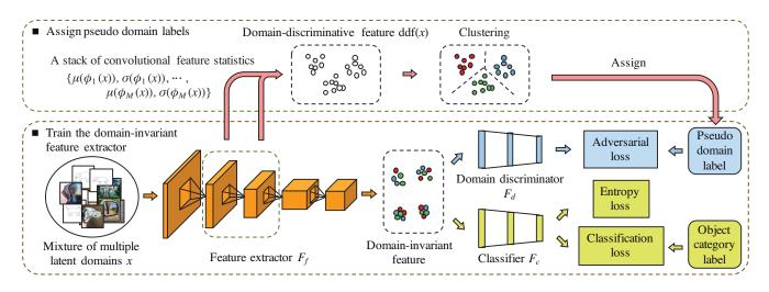
Figure 2: Illustration of our proposed method: Our method iteratively assigns pseudo domain labels by clustering domaindiscriminative features extracted from lower layers of the feature extractor, and trains the domain-invariant feature extractor via adversarial learning.
