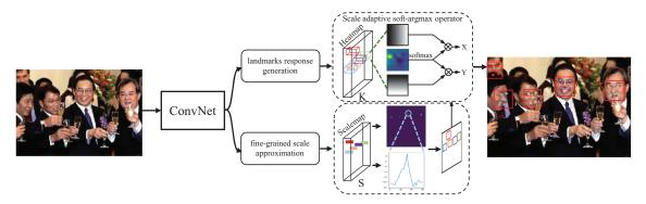
Figure 2: Overview of KPNet. The backbone is followed by two specific modules, one for generating the landmarks response map and the other for approximating the fine-grained face scale. Utilizing the predictions from both modules, the landmarks extractor locates the facial keypoints and infer the face boxes. K and K0 represent the channel numbers of the feature maps.
