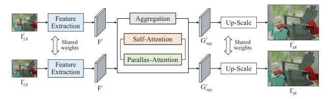
Figure 2: The architecture of proposed method. Stereo images are fed into the feature extraction part for generating highly discriminative features to find stereo correspondence. Then, the feature aggregation part produces view-symmetric and rich informative features for stereoscopic SR using a self and parallax attention mechanism (SPAM). The up-scale part outputs the SR image of each view.
