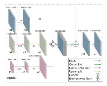
Figure 3: Illustration of the detail implementation of a FPM block with a residual connection, which is formally formulated by Eq. 1. This is an example of N=5, k=3, i.e. FPM1-3 and FPM2-3 in Fig. 2.
