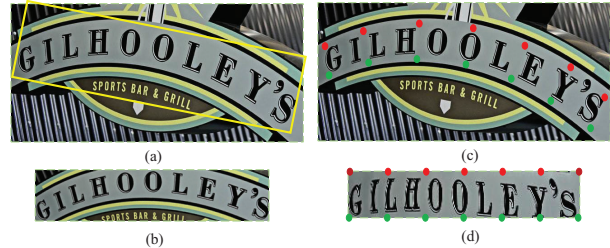
Figure 1: Illustrations of two kinds of methods for text region representation. (a) An oriented rectangle box is used to represent the text region and cropped as (b); (c) A set of boundary points are used to represent the text region, and it can be transformed into a horizontal region like (d).
