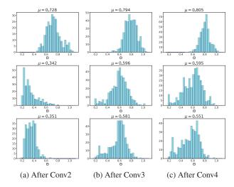
Figure 4: The histogram of  $\theta$  for trainable binarization functions after convolution layers in AlexNet. Three rows, from top to bottom, correspond to  $\rho=0.1,0.3,1.0$  respectively.  $\mu$  is the mean value of  $\theta$  across different channels (each channel has its own  $\theta$ ). Shallow layers require dense representation while deeper layers tend to have higher sparsity.
