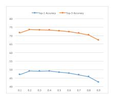
Figure 3: The accuracy on AlexNet for different sparse thresholds ranging from 0.1 to 0.9, which is consistent with the mutual information loss in Figure 2.
