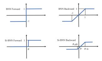
Figure 1: Forward and backward functions for BNN and Si-BNN. Our approach utilizes sparse representation instead of dense predictions in previous methods. Both  $\theta$  and  $\Delta$  are trainable parameters to adaptively deactivate activations and gradients.  $\rho \in [0,1]$  is the hyperparameter, which allows more gradients propagate through activated neurons (i.e., +1 neurons in forward propagation).
