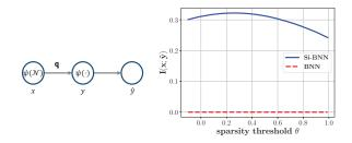
Figure 2: Mutual information between x and  $\hat{y}$  in a minimal model. (Left) A three neuron binarized neural network where Gaussian inputs x after binarization, multiplied by weight  $\mathbf{q} \in \{-1, +1\}$ , and feeds through the same binarization  $\psi(\cdot)$  yielding  $\hat{y}$ . (Right) Mutual information between x and  $\hat{y}$  for different sparsity thresholds.
