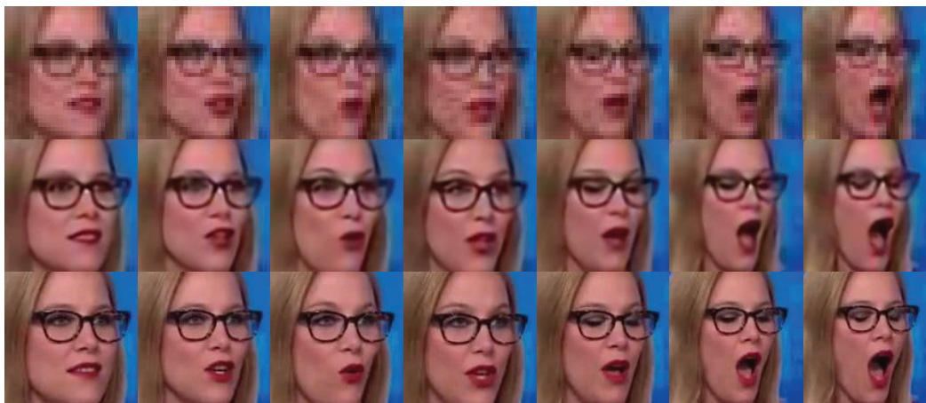
Figure 1: Our method aims to generate high-resolution video frames (2nd row) from low-resolution ones (1st row, visualized using pixel duplication). The low-resolution frames (1st row) are downsampled from the corresponding groundtruth frames (3rd row) with noise and blur.
