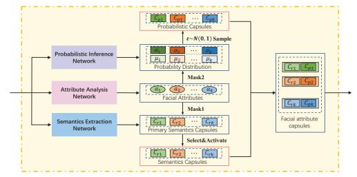
Figure 3: Structure of Capsule Generation Block. The probabilistic capsules are sampled from the posterior using the reparameterization trick with a mask to indicate the present entities. Semantic capsules also be selected and activated by adding masks.
