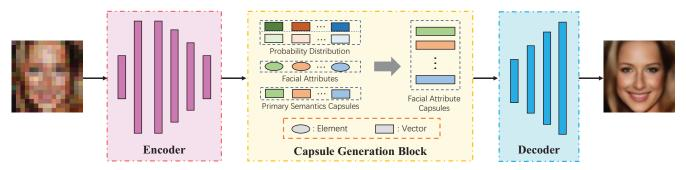
Figure 2: Pipeline of our proposed FACN model. The network consists of two parts: an Encode model to map an input image x into the deep features, a Capsule Generation Block converts the features to a group of facial attribute capsules, and a Decode model to produce the output image  $\hat{y}$  from the facial attribute capsules.
