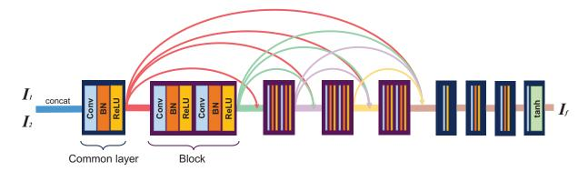
Figure 4: Architecture of the densely connected network (DenseNet). BN: batch normalization. ReLU/tanh: activate function.
