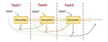
Figure 5: Intuitive description of data flow between different tasks and the process of EWC. Thin lines indicate that only a small subset of data are kept, which are merely used to calculate  $F_i$  and not applied to train DenseNet.
