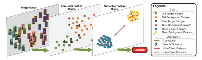
Figure 2: An overview of online-training stage of proposed tracker. We evaluate the training samples in the low-level feature space via the proposed neighbour proximity and eliminate the redundant samples to obtain more informative training set. In semantic feather space, we propose statistic-based losses to obtain more discriminative features for the classifier.
