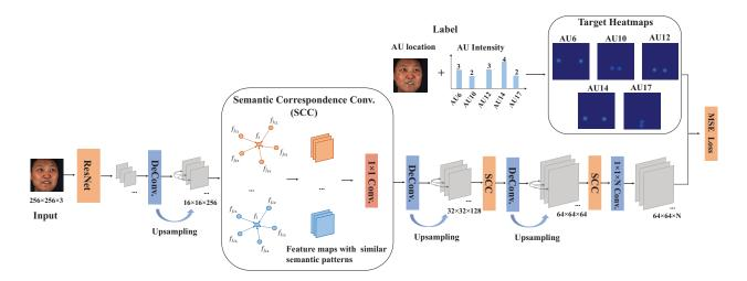
Figure 3: Overview of the proposed pipeline for AU intensity estimation. Given the input face image, the outputs are a set of heatmaps for inferring the intensity level of each AU. The ground-truth heatmaps are generated using the Gaussian function determined by AU locations and the corresponding intensities. The semantic correspondence convolutions are integrated to group feature maps sharing similar semantic patterns and to gradually update the relationship graph layer by layer.
