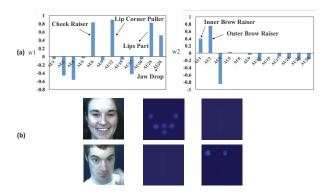
Figure 7: (a) Weights w of the first two feature channels in the last SCC layer corresponding to the output maps. (b) From left to right: Input images; Responses of the first feature channel; Responses of the second feature channel.
