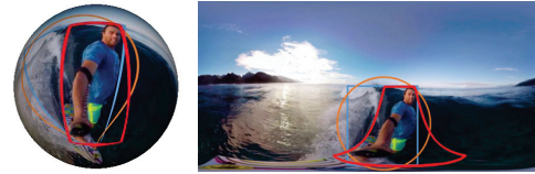
Figure 2: ERPBB (blue outline), CirBB (orange outline) and UnbBB (TanBB/SphBB, red outline) on sphere and ERP.
