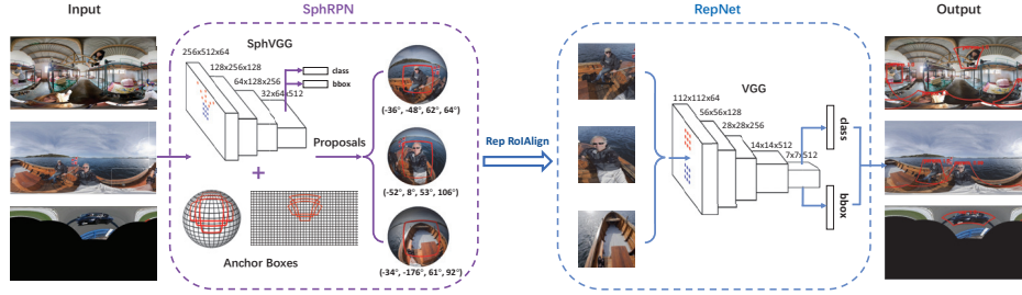
Figure 4: Architecture of Rep R-CNN: SphRPN employs SphRPN to generate coarse proposals; RepNet in the second stage applies a standard VGG backbone and yields precise SphBBs. A Rep RoIAlign layer is applied to bridge SphRPN and RepNet.
