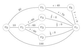
Figure 1: Example with pitfalls for OMT, HOP and ORO. Edge labels p: w denote blocking probability p (omitted for guaranteed roads, i. e., when p = 0) and travel cost w.
