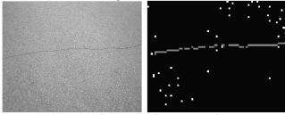
Figure 1. ACE results of a pavement image.
