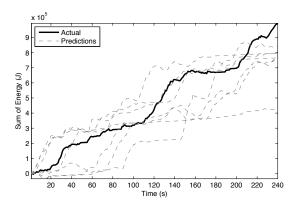
Figure 2: Example set of predictions of upcoming duty versus actual ground truth. Uncertainty can arise from traffic, time delays, or even alternate routes.
