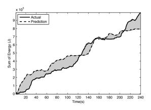
Figure 3: Error calculation for a duty prediction. Shaded area represents error.
