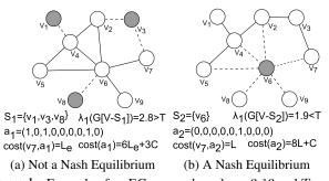
Figure 1: Example of an EC game where  $\lambda_1 = 3.13$  and T = 2. (a) Strategy profile  $\mathbf{a}_1$  where three nodes are secured but spectral radius of the attack graph is more than T = 2; (b) Strategy profile  $\mathbf{a}_2$  where one node ( $v_6$ ) is secured and spectral radius of the attack graph is below T, is a NE. For  $\mathbf{a}_1$ , the epidemic is likely to last long while for  $\mathbf{a}_2$ , the epidemic dies out quickly.
