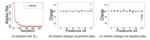
Figure 1: Training-set attack on SVM. The "alcohol" feature is marked by a red star in (b,c).
