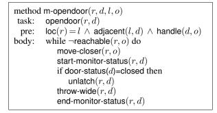
Figure 3: A refinement method for the "open door" task in Fig. 2. The "pre" line gives the method's preconditions, and the body is a simple program to generate a task refinement.
