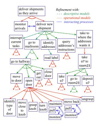
Figure 2: Tasks and actions for a service robot.
